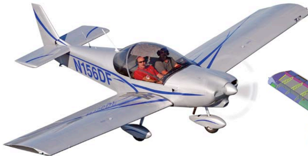
The CH 650 is the most advanced version of Zenith's low-wing clan; it features a taller canopy and revised aerodynamics.
