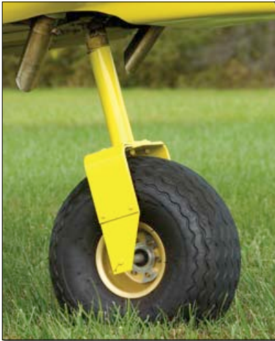
All of the Zeniths have steerable nose-wheels with flotation tires.
