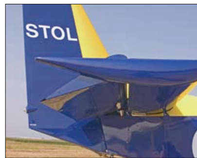
All high-wing Zenith designs have dramatically cambered horizontal stabilizers for improved pitch authority at vanishingly low airspeeds.
