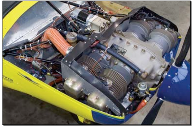
Although the CH 750 flown for this report was fitted with a Jabiru 3300, one option for the design is the Continental O-200.
