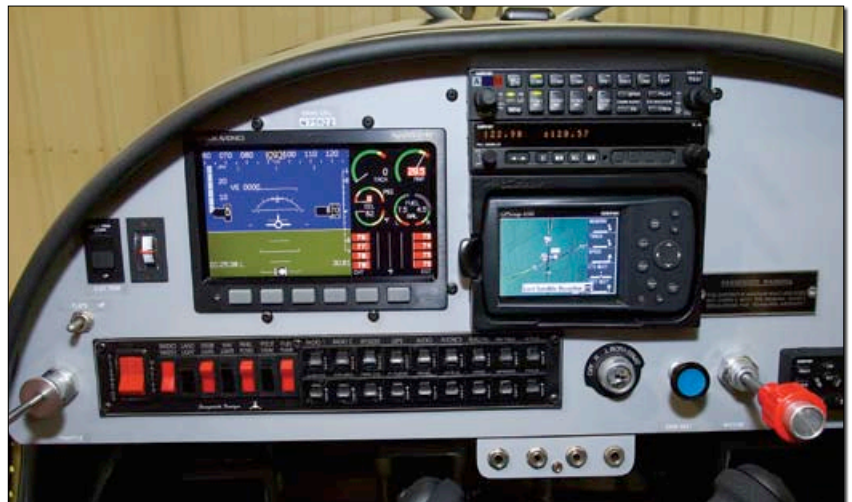
The CH 750's panel is generously sized; the company demonstrator has a Dynon Flight-DEK-D180 combined EFIS and engine monitor.
